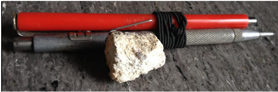
Figure 12 Specimen of the clay-altered/argillized tuffaceous sandstone.
