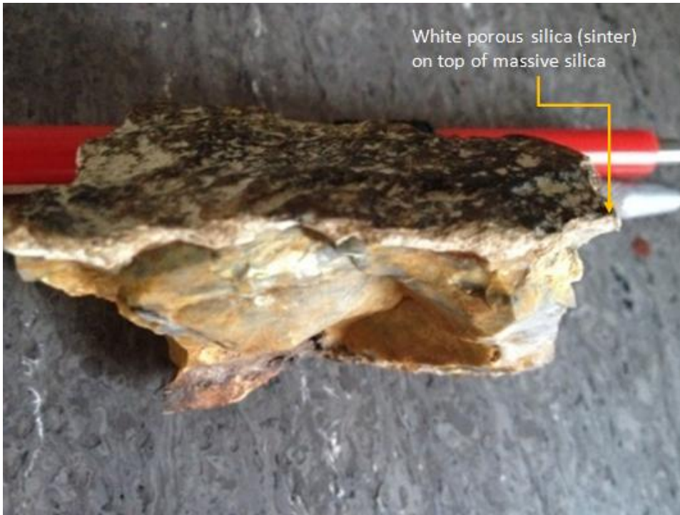
Figure 8c. Sample of the silica with white incrustation of porous silica (sinter) on top.
