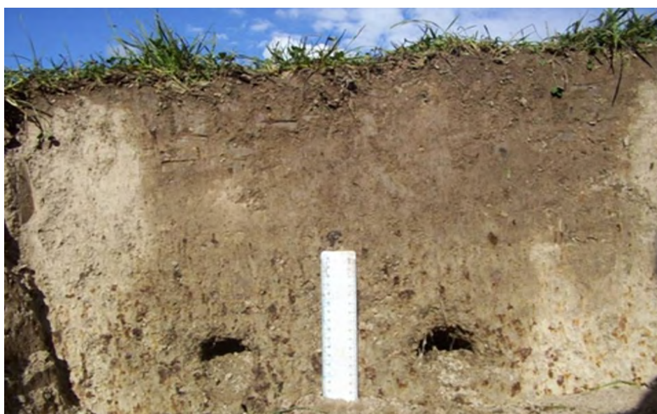
Figure 5. Field example of preferential flow through a Pallic soil containing remnants of old mole drains.
