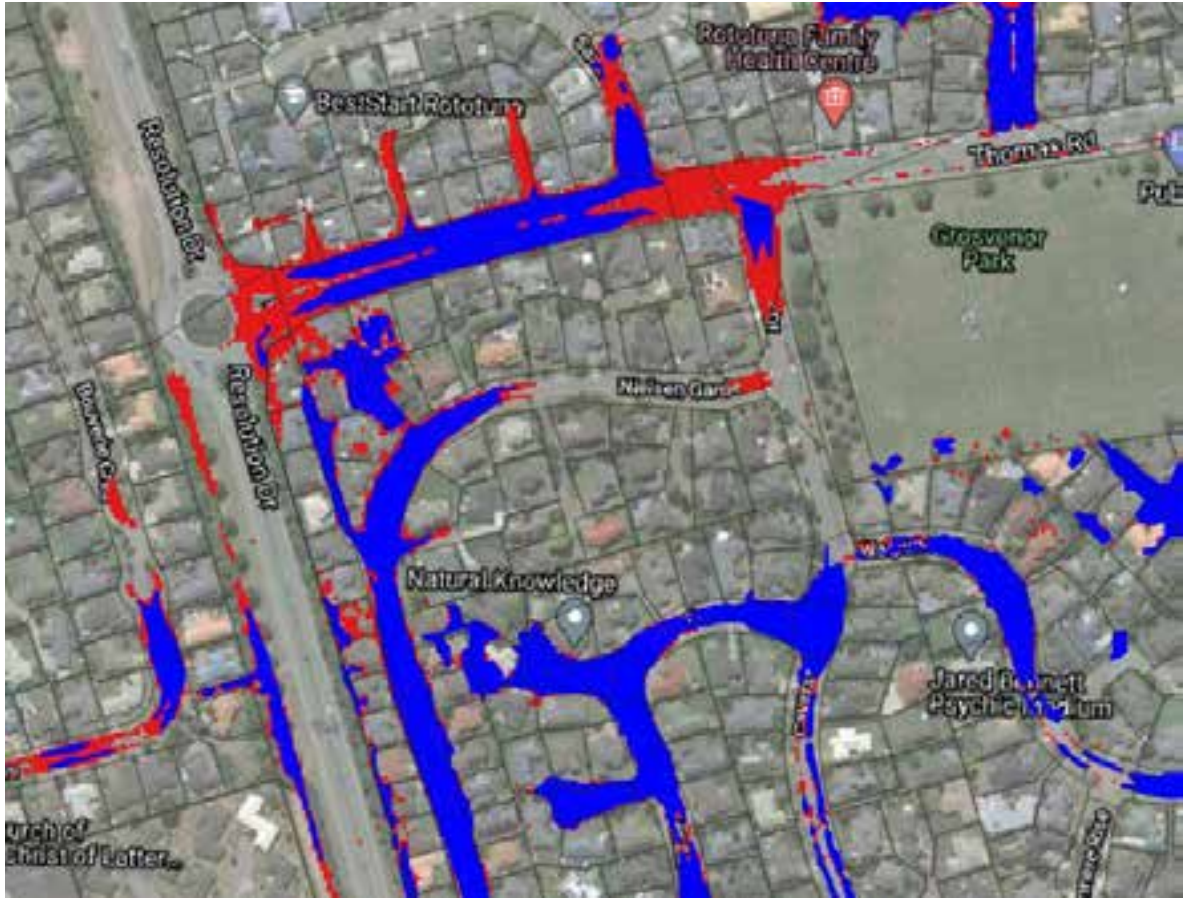
Figure 8 Flood hazard extents at the intersection of Resolution Drive and Thomas Road. ED+CC results shown in blue (2015 model), MPD+CC results shown in red (2017 model).
