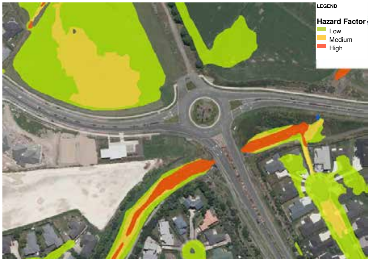
Figure 5 Hazard classifications for the 100 year existing scenario at the Borman Road underpasses
