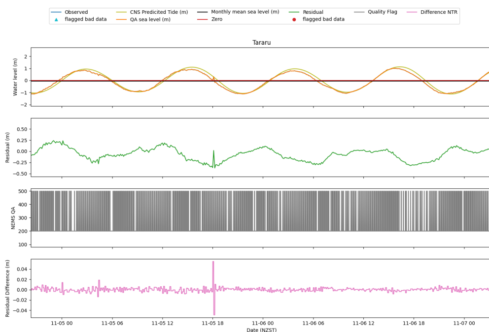
Figure D-5: Spike in Tararu sea-level record which was not detected by the running window filter. Top Pane: Blue raw sea-level data, yellow predicted tide from CNS harmonic fit, orange processed QA sea level. Second Pane: Green non-tidal residual (NTR). Third Pane: grey NEMS QA code. Bottom Pane: Pink, difference in NTR used to identify data spikes.
