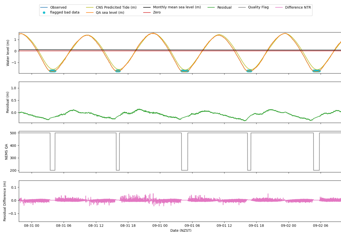
Figure D-3: Stuck values automatically identified between 31/08/2008 and 02/09/2008 in the Raglan raw sea level data. Top pane: yellow line is the predicted tide, orange line QA sea level data, blue dots show the “stuck” raw sea level data. Second pane: green line shows the non-tidal residual (NTR). Third pane: grey line shows the NEMS values. Bottom pane: pink line representing the difference/change in the NTR.
