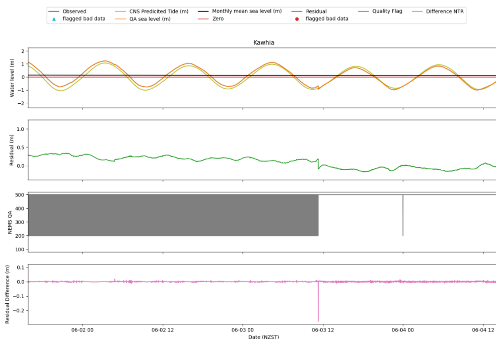
Figure D-6: Datum offset issue identified in the Kawhia sea-level record. Top Pane: Blue raw sea-level data, yellow predicted tide from CNS harmonic fit, orange processed QA sea level. Second Pane: Green non-tidal residual (NTR). Third Pane: grey NEMS QA code. Bottom Pane: Pink, difference in NTR used to identify data spikes.
