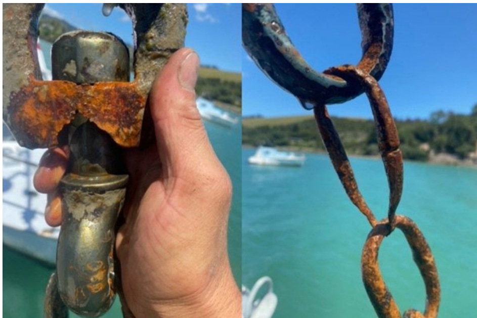
Hardware from a mooring where the owner couldn't show an up-to-date inspection certificate, meaning this hardware could be up to 6 years old. If it had failed, they most likely wouldn't have been covered by their insurance, creating an expensive problem for the owner.
