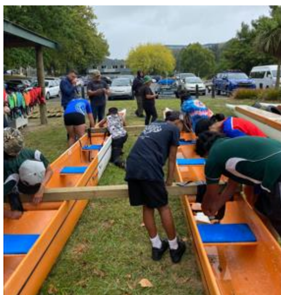
Figure 8: Tauira rigging the waka using aukaha.
