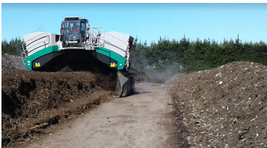
Figure 3-12 Open Windrow Composting with a specialist windrow turner (Waste Management 2018)
