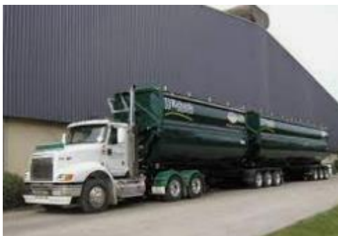
Figure 3-6: Double haulage vehicle for transporting liquid or semi-liquid material (J.J. Richards & Sons Pty Ltd n.d.)
