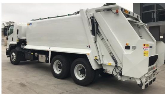
Figure 3-3: Example rear loader (Waste Management Review 2020)
