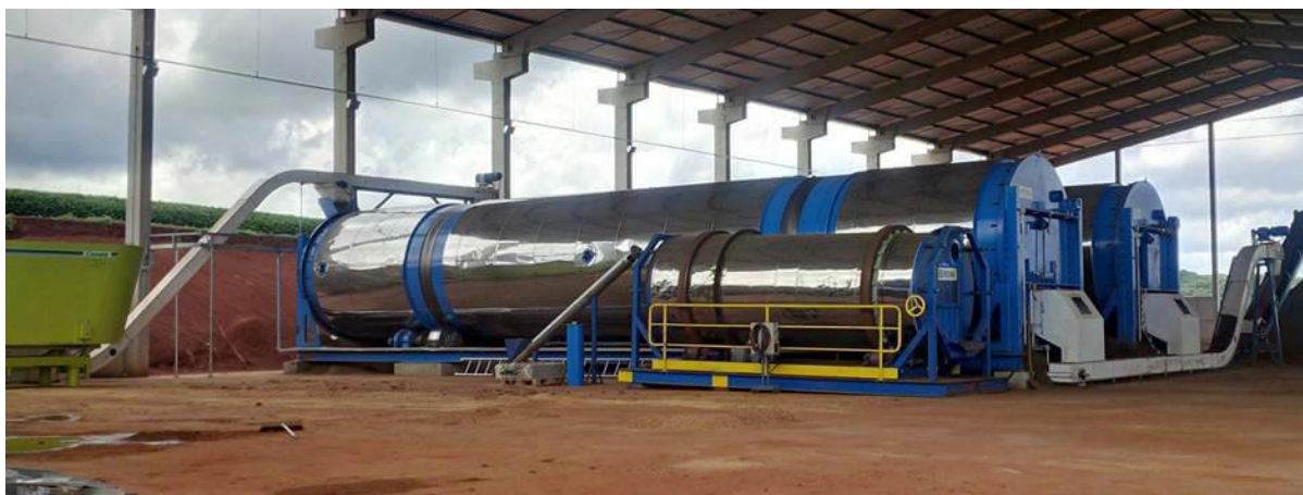
Figure 3-13: In-vessel Composting System (X-Act Systems N.D.)
